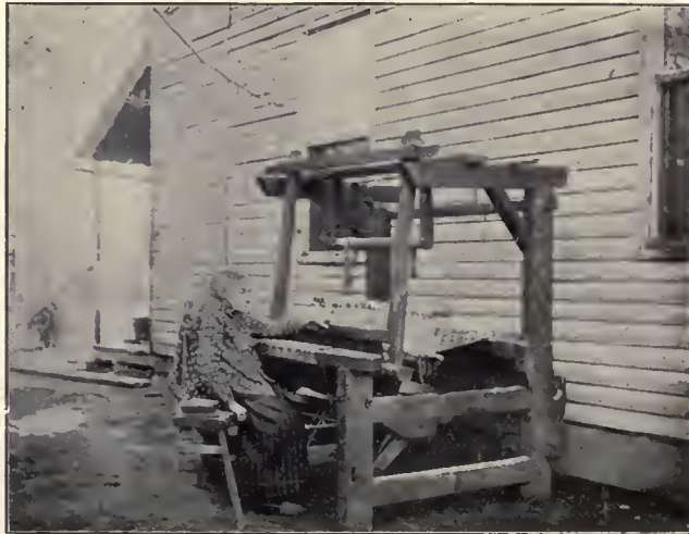
A HOME-MADE LOOM USED IN WEAVING CARPETS
